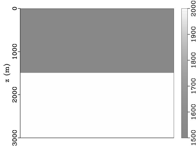
Figure 1: The 1.5D two half-space homogeneous velocity model I used in the example.
