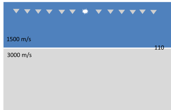
Figure 6: A discontinuous velocity model used to propagate the wavefield. There is one reflector at 110 m, the velocities are 1500 m/s and 3000 m/s above and below the reflector, respectively.
